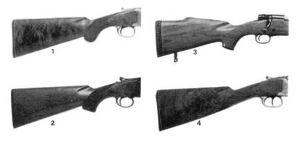
Fig. 2.10 - Stock type - 1. Semi Pistol, 2. Pistol type, 3. Monte Carlo, 4. English type
